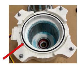
to this fact, we cannot provide a serial number range of equipment containing motors with the O-ring seal. The only way to identify this is by motor date code.
